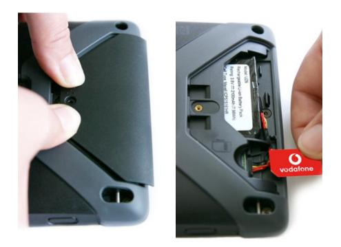
**3.** Push the lid of the battery compartment to the side and detach it from the PRO 8275.
