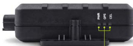
Power LED / GPS LED / CEL LED
